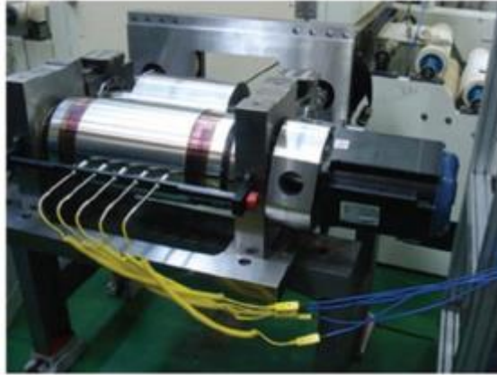
Figure 2.18: A setup of R2R system with an induction heating coil inside the heating roller
