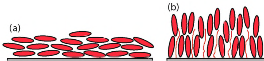
Figure 2.3: Cartoon of different orientations of liquid crystals molecules on interfaces: (a) tangential orientation is also called planar anchoring and (b) orientation normal to the interface is called homeotropic anchoring.
