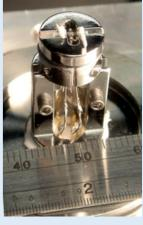
Development of a prototype of a compact QEPAS sensor for the detection of ethylene. Study of the response of the etylene sensor for breath analyis application with gas matrices that simulate human breath. Coupling of the sensor with a breath sampling system and preliminary test with real samples of human breath.
