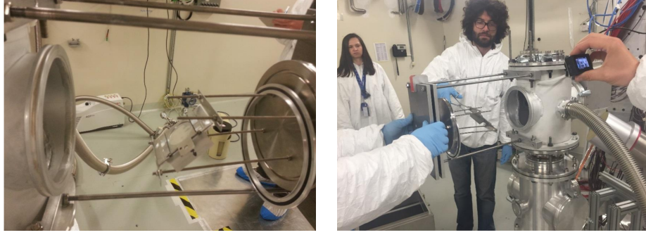
Figure 3.18: Insertion of the ^7\text{Be} sample in the aluminum vacuum chamber.
