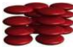
Figure 2.12: Molecules arranged in stacks in the columnar phase.
