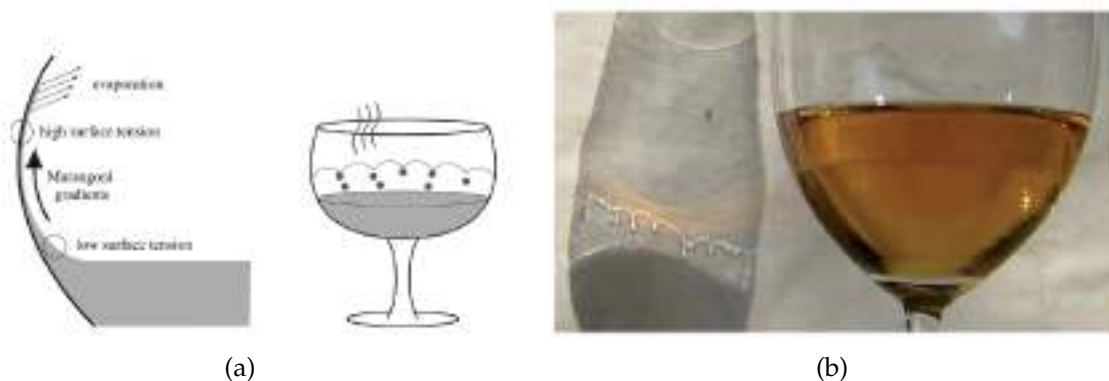
Figure 6.3: Schematic view of the phenomenon of the "tears of wine". When ethanol evaporates from the thinner region of the meniscus, a surface tension gradient is generated and the liquid climbs the glass spontaneously forming a film and then, thanks to gravity, tears. (b) Photo of a glass of wine with the "tears of wine" [145, 146].
