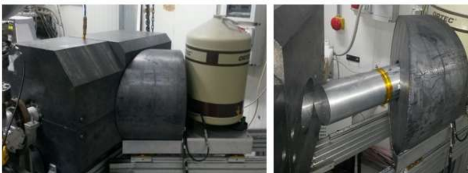
Figure 2.13: Lead shielding in the HPGe configuration.
