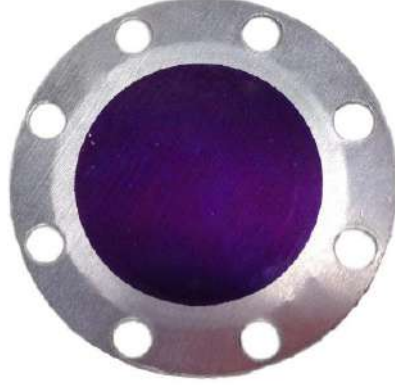
Figure 2.7: Photograph of one of the Ta_2O_5 targets produced before beam exposure.
