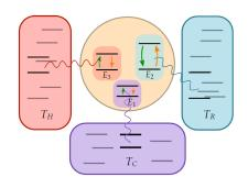
Schematic diagram of a three qubit refrigerator (inside the yellow circle) coupled to three thermal reservoirs.
