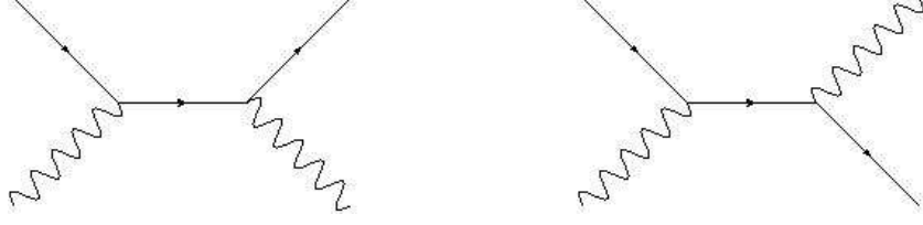
FIGURE 1.10: Feynman diagrams for Inverse Compton Scattering.
