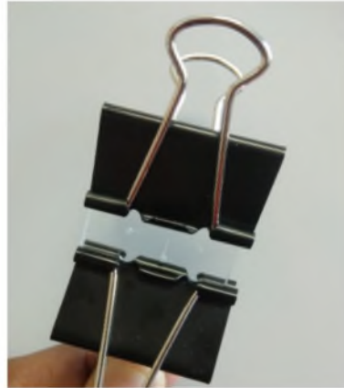
Figure 4: Stacked PMMA slabs with plastic clamp
