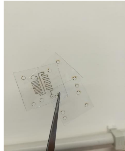
Figure 9: Laser cut microstructures on individual layers
