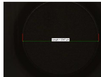
Figure (b) : Bottom diameter(2347 \mu m) of valve with millimeter dimension
