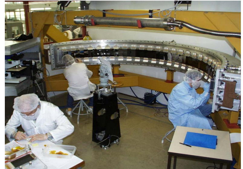
Telescope of 32 MSGCs tested at PSI in Nov99 (CMS Milestone)
