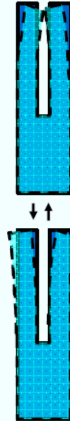
c) vibration mode of tuning fork
