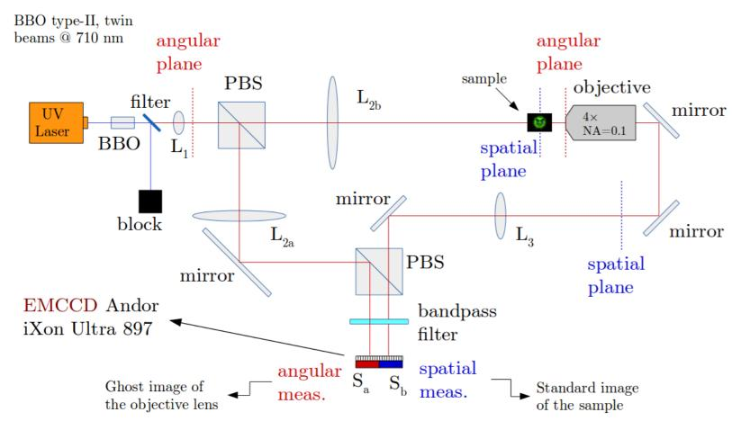
$L_1: reproduces in its focal$ plane ("angular plane") the FTof the signal and idler beams $(f_1 = 10 mm)$
