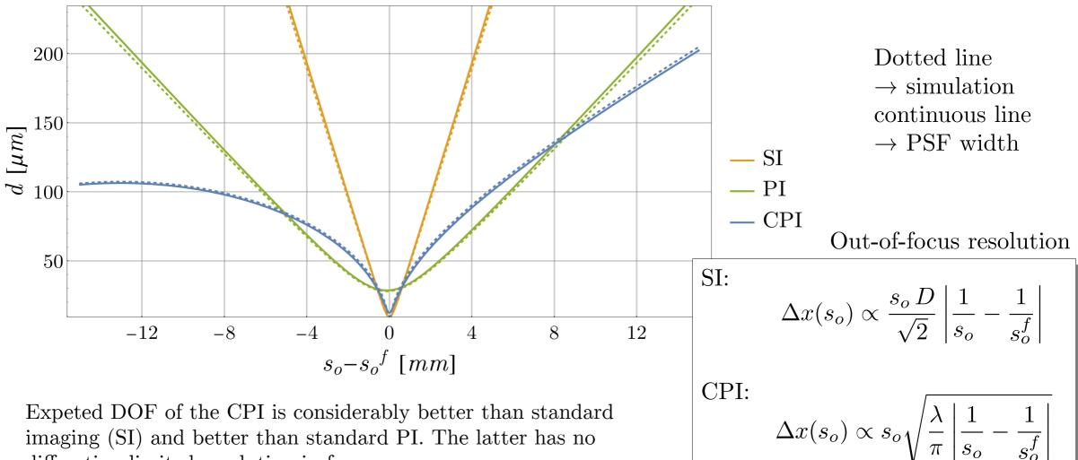
imaging (SI) and better than standard PI. The latter has no diffraction limited resolution in focus.
