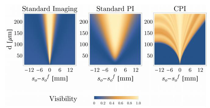
Expected DOF of the CPI is considerably better than standard imaging and better than standard PI. Unlike standard PI the CPI keeps the resolution of standard imaging.
