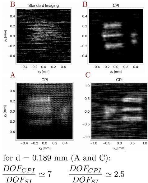
Visibility of the image of a double slit (distance d = 2 width)
