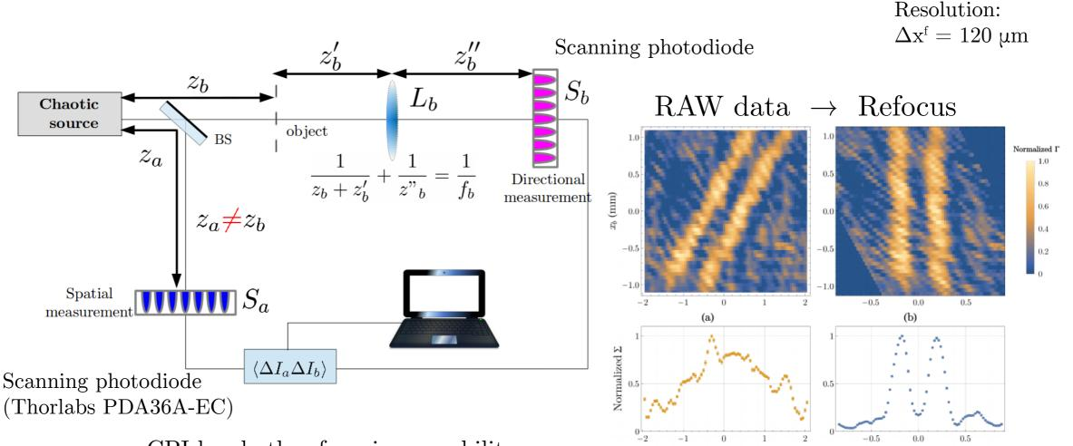
CPI has both refocusing capability and diffraction limited resolution!
